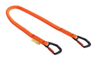
This tool Lanyard features an aluminum auto locking carabiner with a captive eye on both ends to tether tools up to 10kgs. This shock-absorbing lanyard is designed and tested to reduce the force by absorbing the energy transmitted through the tool lanyard.
