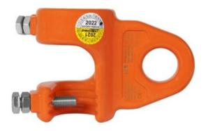
The AT187 anchoring point is a type B anchoring device. It can only be used as personal fall protection equipment and must not be used for lifting cargo. The strength of this point is min.30 kN.The point can be loaded in the directions shown in the figure.The device is designed to be installed on ribbed bars with a core of 18-32 mm in diameter.
