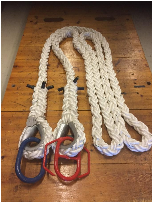
Pennant with master link in one end and ring with handles in other end
