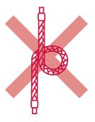
11. Do not kink when lifting The wire sling is damaged and thereby loses strength.
